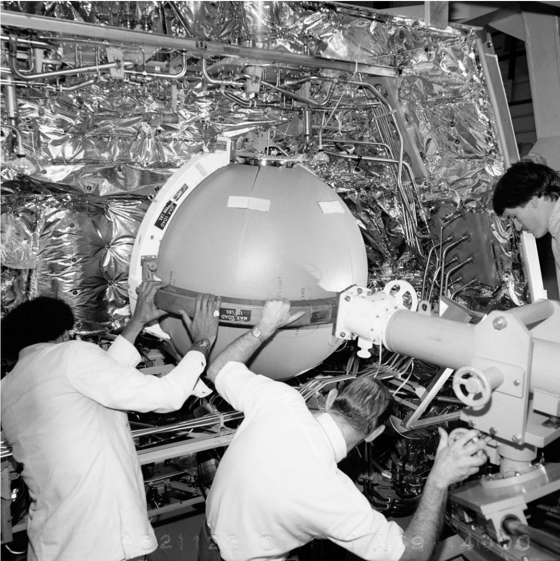
Figure B-14. Fuel tank being installed into Discovery's FRCS module, NAR Building 1, Downey, California, November 23, 1982. Source: NASA, Johnson Space Center Image Repository, JSC2010-03369.
